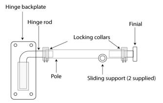
When the hinge backplate is fitted to a doorjamb and the sliding support fitted to a door the pole will open with the door, alternatively the pole can be lifted off the sliding support on the door and swung open and placed on the support on the return wall for times when the curtain is not required over the door
